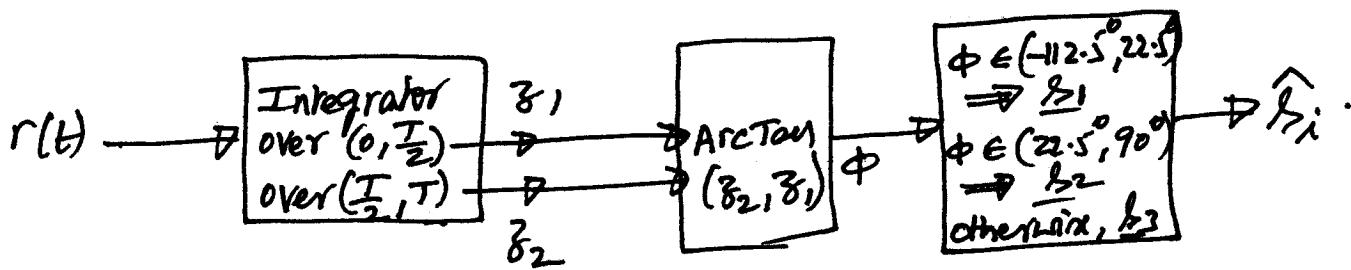
If  $\tan^{-1}(z_2, z_1) = \phi$  is an angle between  $-112.5^\circ$  to  $+22.5^\circ \Rightarrow$  choose  $b_1(t)$
