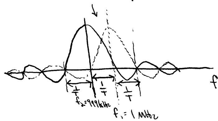
$$\text{total bandwidth} = \frac{2}{T} + \frac{1}{T} = \frac{3}{T} = 3 \text{ KHz}$$
