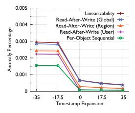
Figure 7: The percentage of reads flagged as anomalies by our checkers for different timestamp expansions for vertices. Expanding timestamps *X*ms subtracts *X* from the invocation time and adds *X* to response time.
