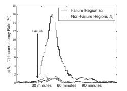
Figure 13:  $\phi(R_i:G)$ -inconsistency for the photo comment type after a misconfiguration. This metric enables us identify the geographic region to which the incorrect configuration was pushed.
