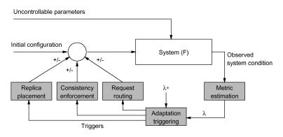
Fig. 3. Interactions between different components of a wide-area replica hosting system.
