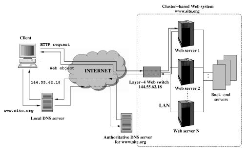
Fig. 7. Layer-4 two-way architecture.
