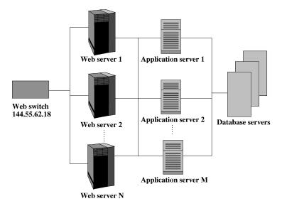
Fig. 17. An example of multitier architecture for a Web cluster.
