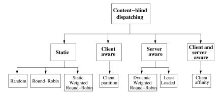
Fig. 15. Content-blind dispatching algorithms.
