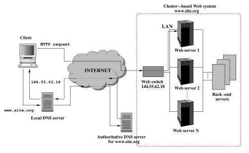
Fig. 3. Architecture of a cluster-based Web system.
