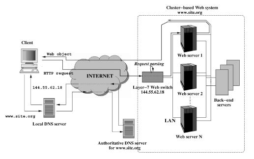
Fig. 11. Layer-7 one-way architecture.
