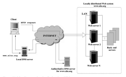
Fig. 2. Model architecture for a locally distributed Web system.
