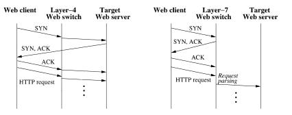
Fig. 9. Operations of layer-4 routing (left) and layer-7 routing (right).
