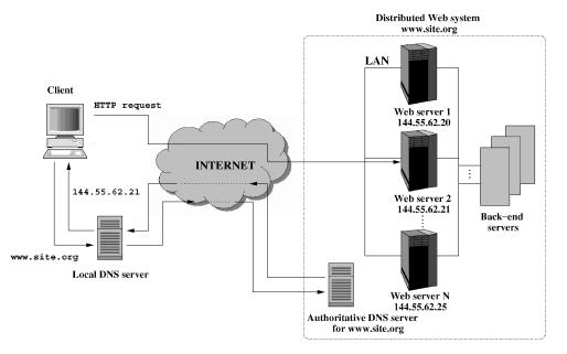
Fig. 5. Architecture of a *distributed Web system*.
