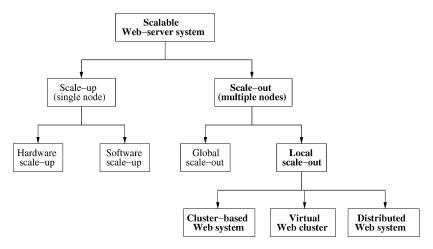
Fig. 1. Architecture solutions for scalable Web-server systems.
