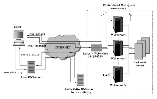
Fig. 8. Layer-4 one-way architecture.
