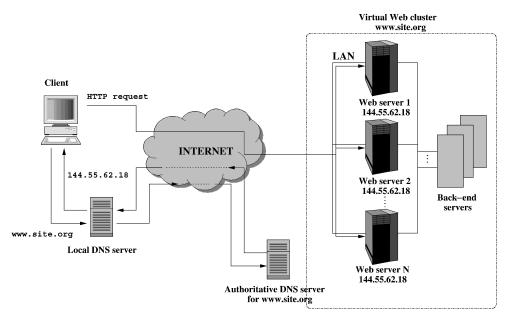
Fig. 4. Architecture of a virtual Web cluster.
