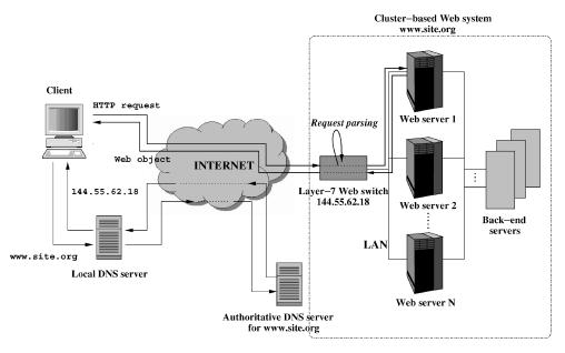
Fig. 10. Layer-7 two-way architecture.
