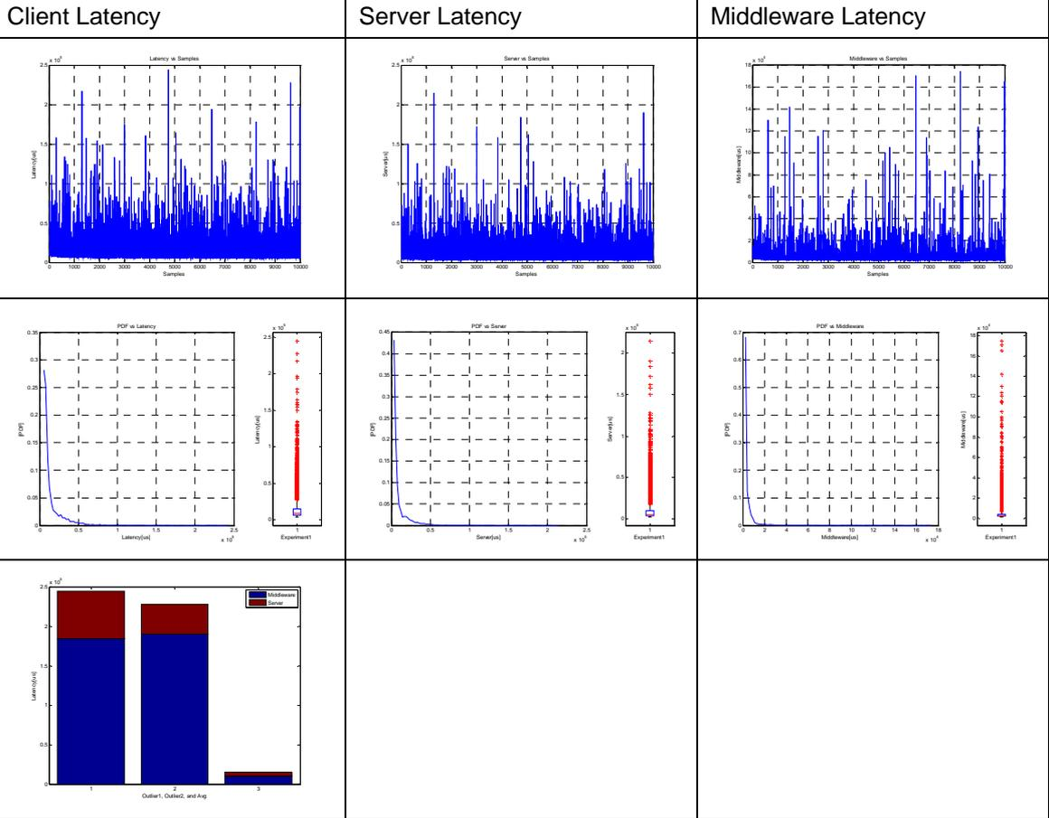
Experiment 12 – # of Client = 1, Size of Reply = 1024byte , Request Time = 40ms
