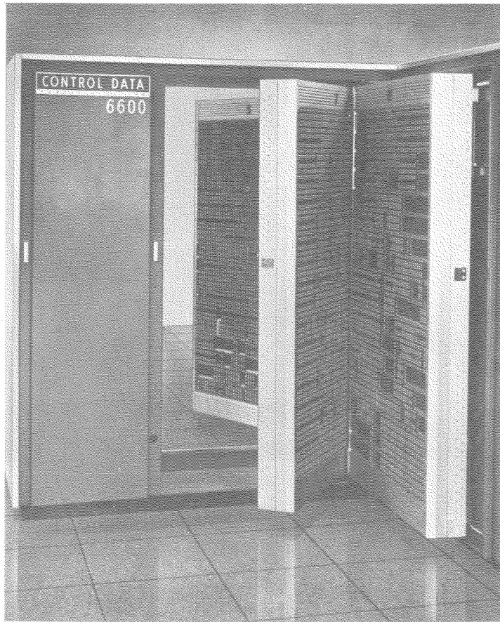
Figure 9. 6600 Main Frame Section.
