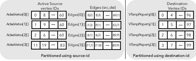
Fig. 8: Data layout for the parallel implementation of Graphiconado.
