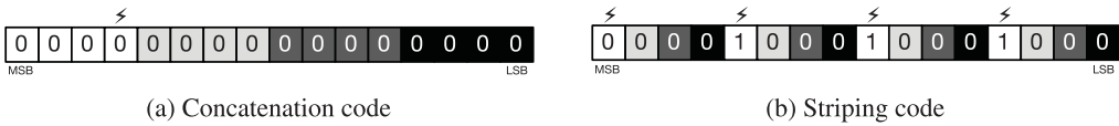
Fig. 4. Two codes for storing 16-bit numbers in four 4-bit cells. Each color indicates a different cell. A single-level error leads to a bit flip in the indicated position. In (a), this is the lowest-order bit in the white cell. In (b), the white cell holds the binary value 0111, which is one level away from 1000.
