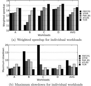
Figure 5. TCM vs. other algorithms for 4 sample workloads and averaged across 32 workloads
