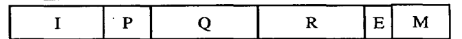
Figure 2. Base Processor's Integer Pipeline. I = IBOX consisting of the thread chooser, line prediction, instruction cache access, and the rate matching buffer. P = PBOX consisting of wire delays and register rename, Q = QBOX consisting of instruction queue operations, R = RBOX consisting of register read stages, E = EBOX consisting of functional units, and M = MBOX consisting of data caches, load queue, and store queue. In our evaluation, we assumed the following latencies: I = 4, P = 2, Q = 4, R = 4, E = 1, and M = 2 cycles.
