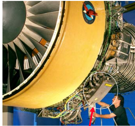
PW-4000 FADEC (Full Authority Digital Engine Controller)
