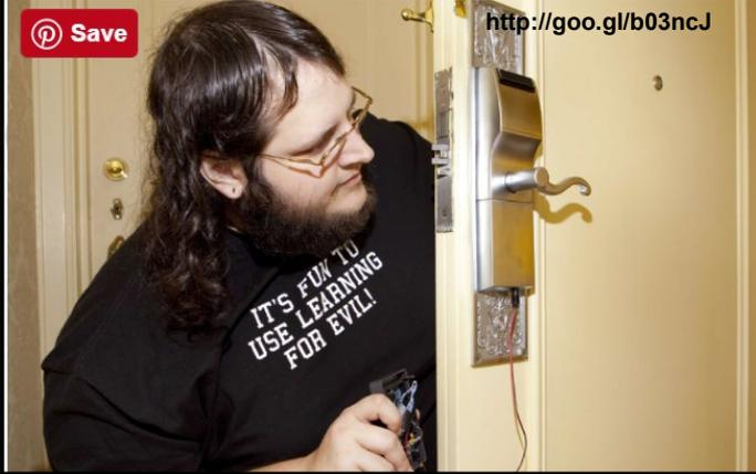
The system's vulnerability arises, Brocius says, from the fact that every lock's memory is entirely exposed to whatever device attempts to read it through that port. Though each lock has a cryptographic key that's required to trigger its “open” mechanism, that string of data is also stored in the lock's memory, like a spare key hidden under the welcome mat.
