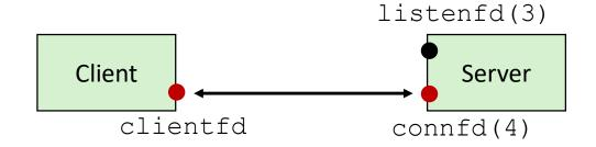
3. Server returns connfd from accept. Client returns from connect. Connection is now established between clientfd and connfd
