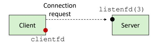
2. Client makes connection request by calling and blocking in connect
