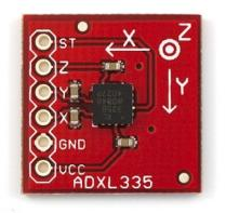
Fig 4.1: ADXL335 Accelerometer
