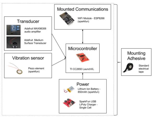
Fig 5.1: Mounted Subsystem Breakdown
