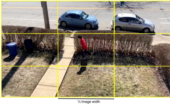
Figure 2: Example target with 3x3 grid overlay. The drone should always try to keep the target within the center rectangle.
