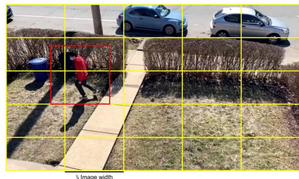
Figure 1: Example target with 5x5 grid overlay. The red bounding box centered around the target has a length of \frac{1}{5} of the camera width.
