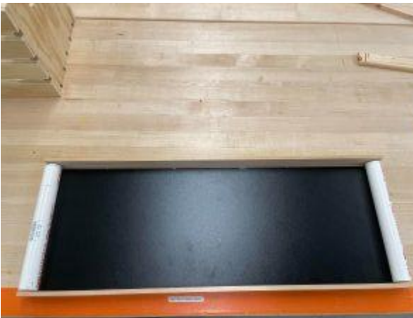
Fig 3. Partially Completed Conveyor Belt System
