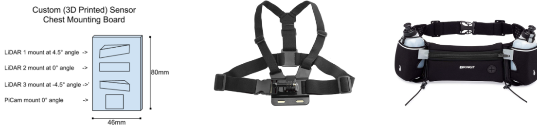
Figure 2: (a) Design for 3D printed mounting board (b) sensor harness (c) hydration belt for battery and Raspberry Pi
