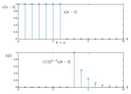
Because the function h[k] does not begin until k = 3, the product of x[n-k] and h[k] will be nonzero only for  $n \ge 3$ , as before. For values of  $n \ge 3$ , the output is computed as
