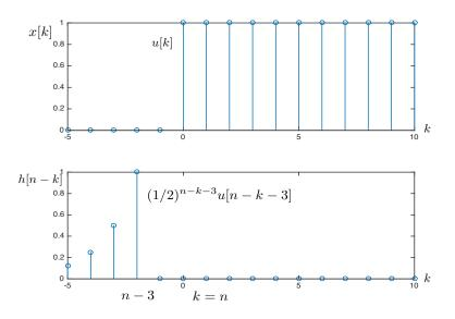
Note that h[n-k] is developed by replacing the *n* in h[n] by n-k wherever it appears. Because the original function,  $h[n] = \left(\frac{1}{2}\right)^{n-3} u[n-3]$ , begins at n = 3, the function h[n-k] ends three samples to the left of the sample k = n. Note also that the two functions x[k] and h[n-k] will have no nonzero overlap at all unless n-3 is greater than zero, or  $n \ge 3$ . For  $n \ge 3$  the sum on *k* will be evaluated for  $0 \le k \le n-3$ .
