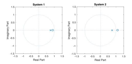
We note that the two systems should have the same magnitude of the frequency response, as System 1 can be obtained by cascading System 2 with an allpass filter with a zero at z = 9/10 and a pole at z = 10/9. And (unsurprisingly) this is the case:
