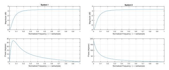
Note that the magnitude of the phase shift is much greater for System 2 than it is for System 1. In general System 1 is preferred over System 2, because it has less phase lag, which is normally considered to be desirable. In the general case, a system is considered to be *minimum phase* if all
