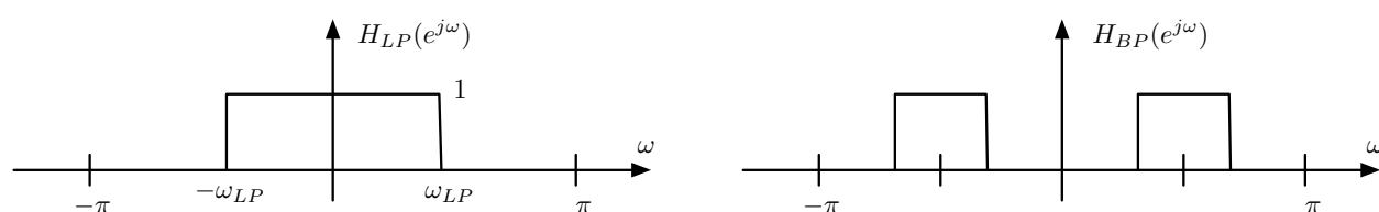
Figure 5a. Ideal lowpass and bandpass filters.
