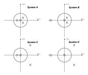
The figure above depict the pole-zero plots of four stable systems. In each case, the poles and zeros have magnitudes that are either 0, 0.5, or 2, and phase angles that are either  $\pm \pi/4$  or  $\pi$  radians. It can easily be shown that the magnitude of the frequency response of all four systems is the same.
