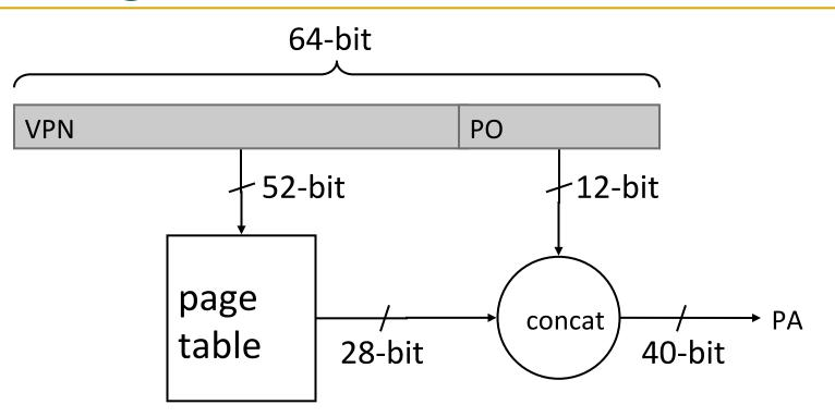
Suppose 64-bit VA and 40-bit PA, how large is the page table?
