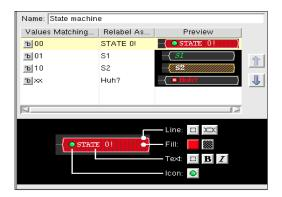
Select the state[1:0] signal in the Waveform Viewer, then press Apply To Selected Signals in the Mnemonic Maps box. (Do this for nextstate, too.)
