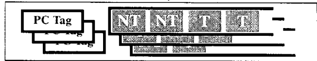
Figure 7. A conceptual view of a control-based prediction correlation mechanism. When a branch is fetched by the main thread, its PC is compared to the correlator's PC tags. If a match occurs, the prediction at the head of the queue overrides the traditional branch predictor.
