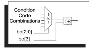
Figure 7. Condition Code Logic Using Mux
