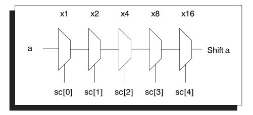
Figure 1. Structured Shift Right Arithmetic Design
