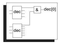
Figure 3. Balanced Tree Decoder
