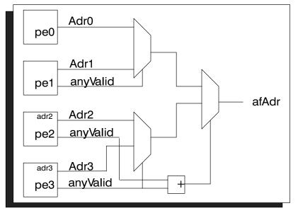
Figure 2. 32-Bit Fast Priority Encoder
