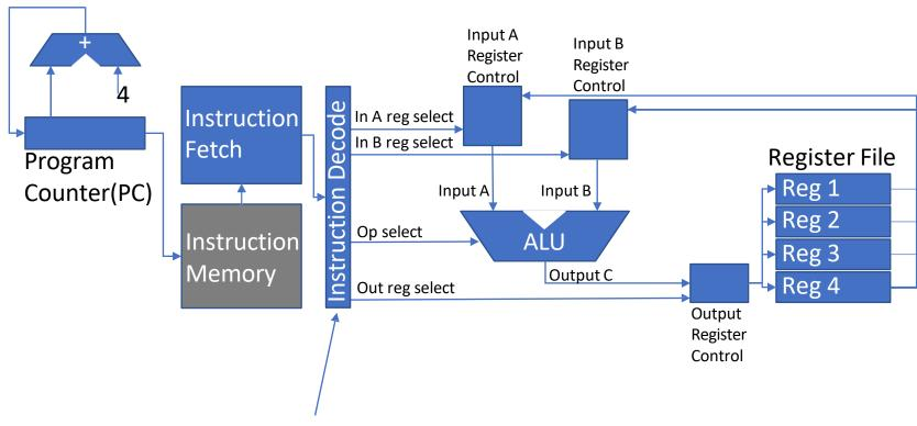
**Instruction** gets decoded into signals that control the other parts of the system (more on encoding / decoding in a few slides)
