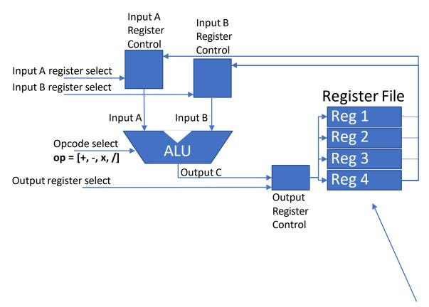
Stateful Elements plus control required to access them, providing inputs to operations and storing outputs of operations
