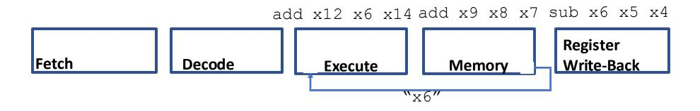
We can *forward* the value in the MEM/WB pipeline register from the sub back to Execute to act as the input operand for the add (going around the unrelated operation in the memory stage)
