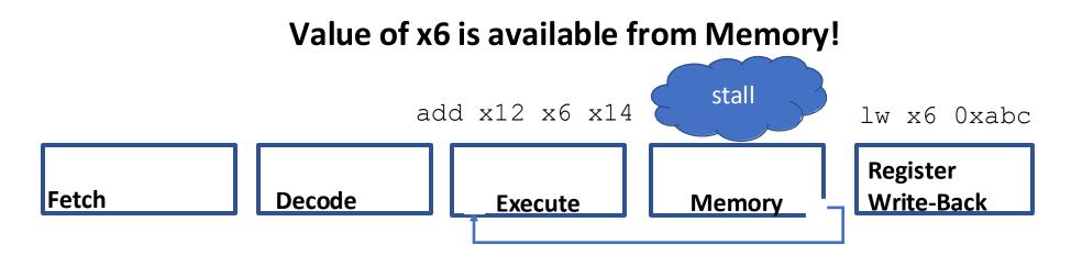
We can *forward* the value in Memory's pipeline register from the lw back to Execute's input for the add
