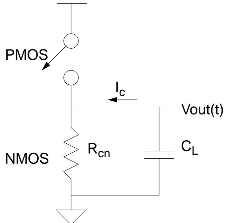
NMOS non-saturated:  $0 < V_{out} \leq V_{DD} - V_{tn}$
