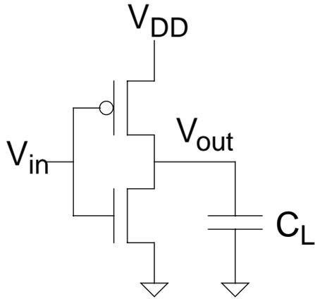
NMOS trajectory:  $V_{out}$  falling.
