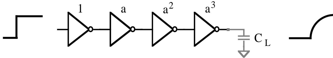
$$\begin{aligned}t_{dr} &= R(2aC) + \\ &\quad (2R/a)(2a^2C) + \\ &\quad (R/a^2)(2a^3C) + \\ &\quad (2R/a^3)(C_L) \\ &= 8RaC + 2RC_L/a^3\end{aligned}$$
