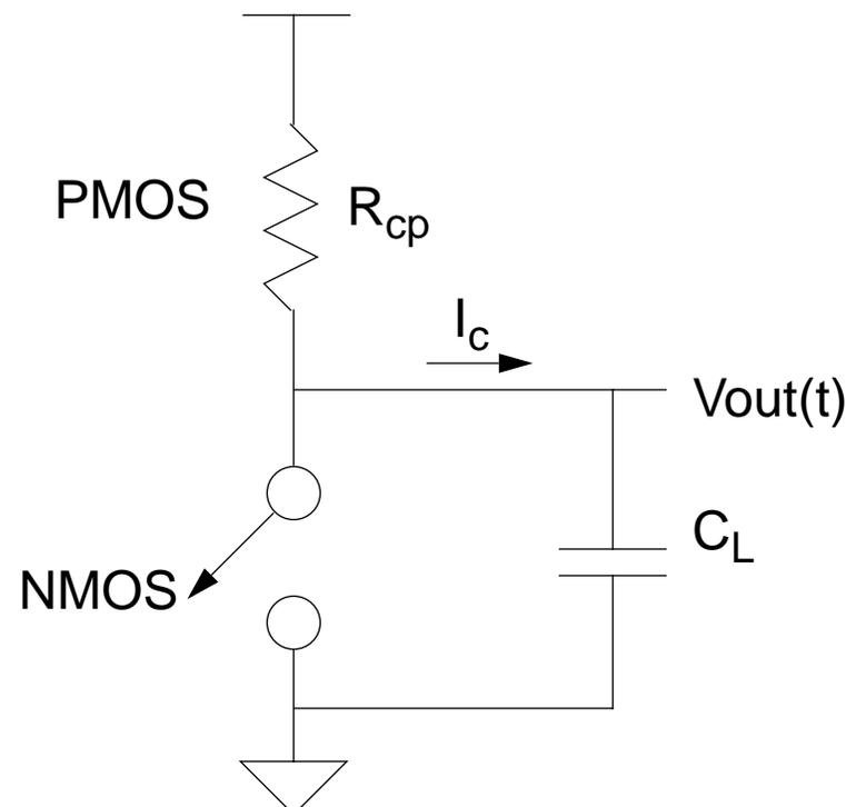
PMOS non-saturated:  $|V_{tp}| < V_{out} < V_{DD}$
