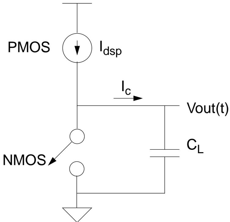
PMOS saturated:  $V_{out} \leq |V_{tp}|$
