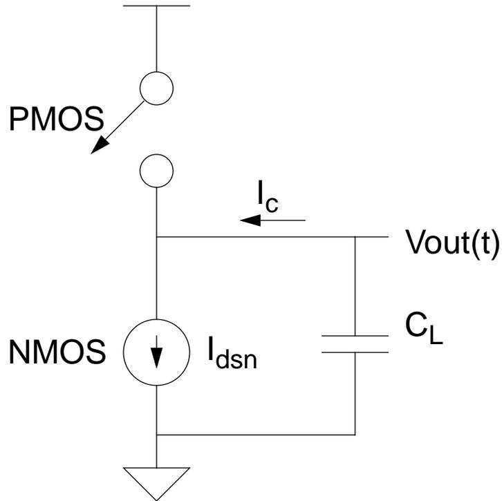
NMOS saturated:  $V_{out} \geq V_{DD} - V_{tn}$
