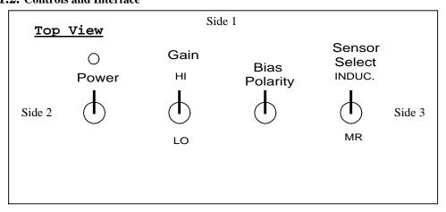
One can see from above the control unit for the device. Use these switches to operate the device as described below.
