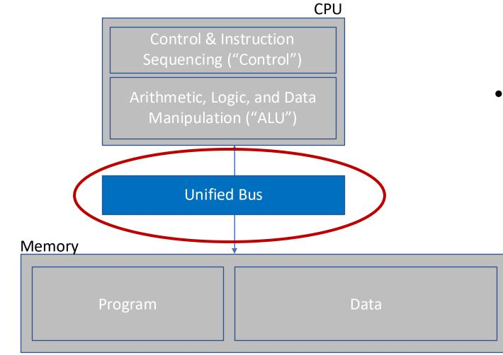
• Data & Program share a bus into the CPU. Need to time multiplex access to the bus.
