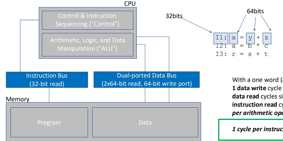
With a one word (8 byte) bus: 1 data write cycle simultaneous with 1 data read cycles simultaneous with 1 instruction read cycle per arithmetic operation
