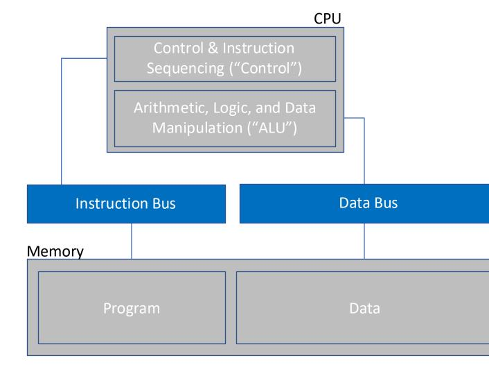
Split bus architecture provides *simultaneous* access to program and to data
