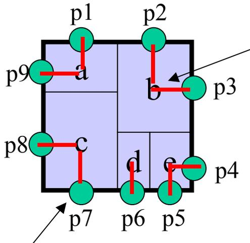
Create another wire from each pin to the center of the block it touches. Note, each pin is on just one wire.
