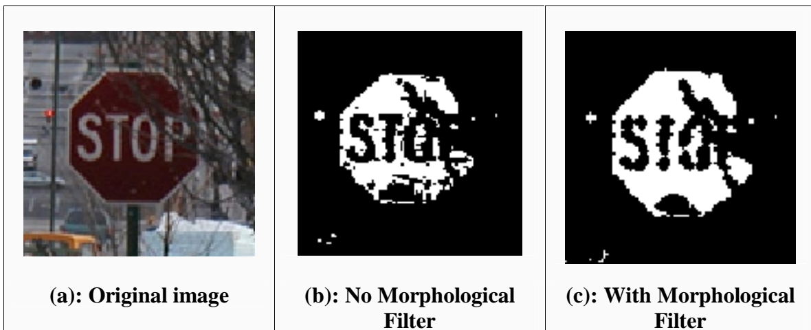
Figure 3: Differences in output obtained when using a morphological filter.
