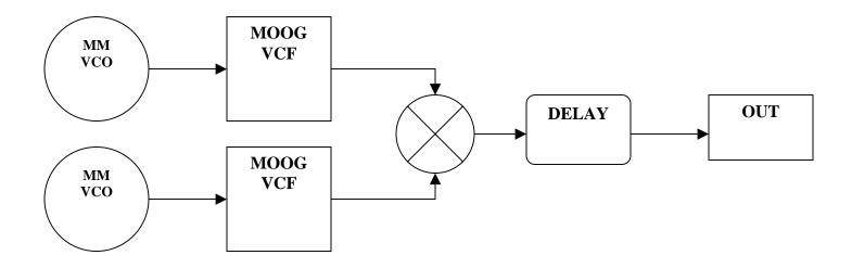
Configuration involving two oscillators (Usually an even and an odd harmonic generator) that are mixed after filtration, with delay added to give some reverb. This configuration is great for making organ tones.
