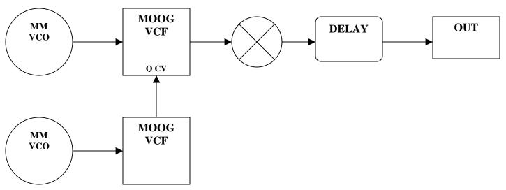
Dual oscillator configuration with the second oscillator modulating the resonance of the filter that takes the first oscillator as an input. Great for making metallic sounds, such as cymbals.
