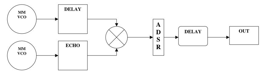
Dual oscillator configuration with independently controlled delay and echo paths for each oscillator. This yields a different beat frequency for each harmonic set. Great for analog modeling of higher order distortion effects, or creating heavy vibrato.
