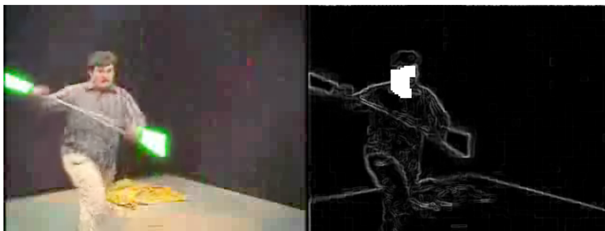
Figure 3.4: Input frame and resulting face detection output (with primitive edge detection shown as a guide)
