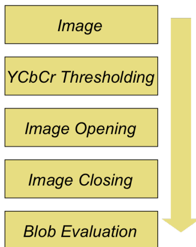
Figure 3.3: Face detection block diagram
