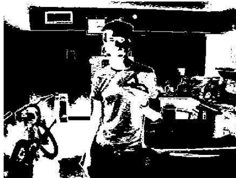
Figure 25: Thresholding without White Balance
