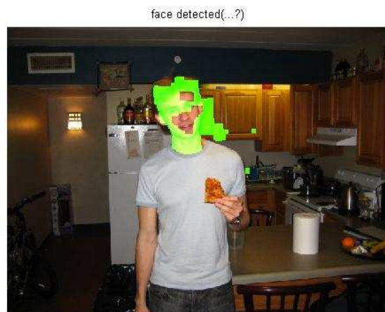
Figure 28: Thresholding with White Balance
