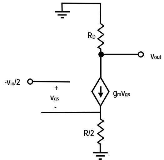
Fig. 4 – Half-Circuit Small Signal Model
