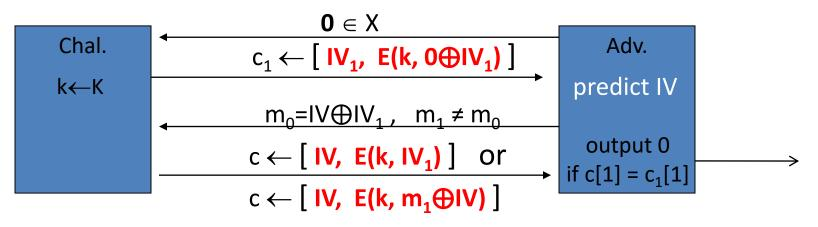
Bug in SSL/TLS 1.0: IV for record #i is last CT block of record #(i-1)
