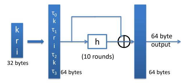
h: invertible function. designed to be fast on x86 (SSE2)
