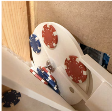
2) Chip hopper puts chips into line
