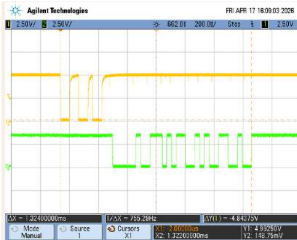
Figure 8: Oscilloscope Output for MIDI Latency Test
