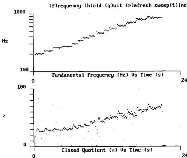
FIG. 3. A plot of a two-octave ascending G major scale sung by a trained subject (F11):  $\log(F_0)$  against time (upper), and closed quotient measured by method (a) of Davies et al. (21) against time (lower).
