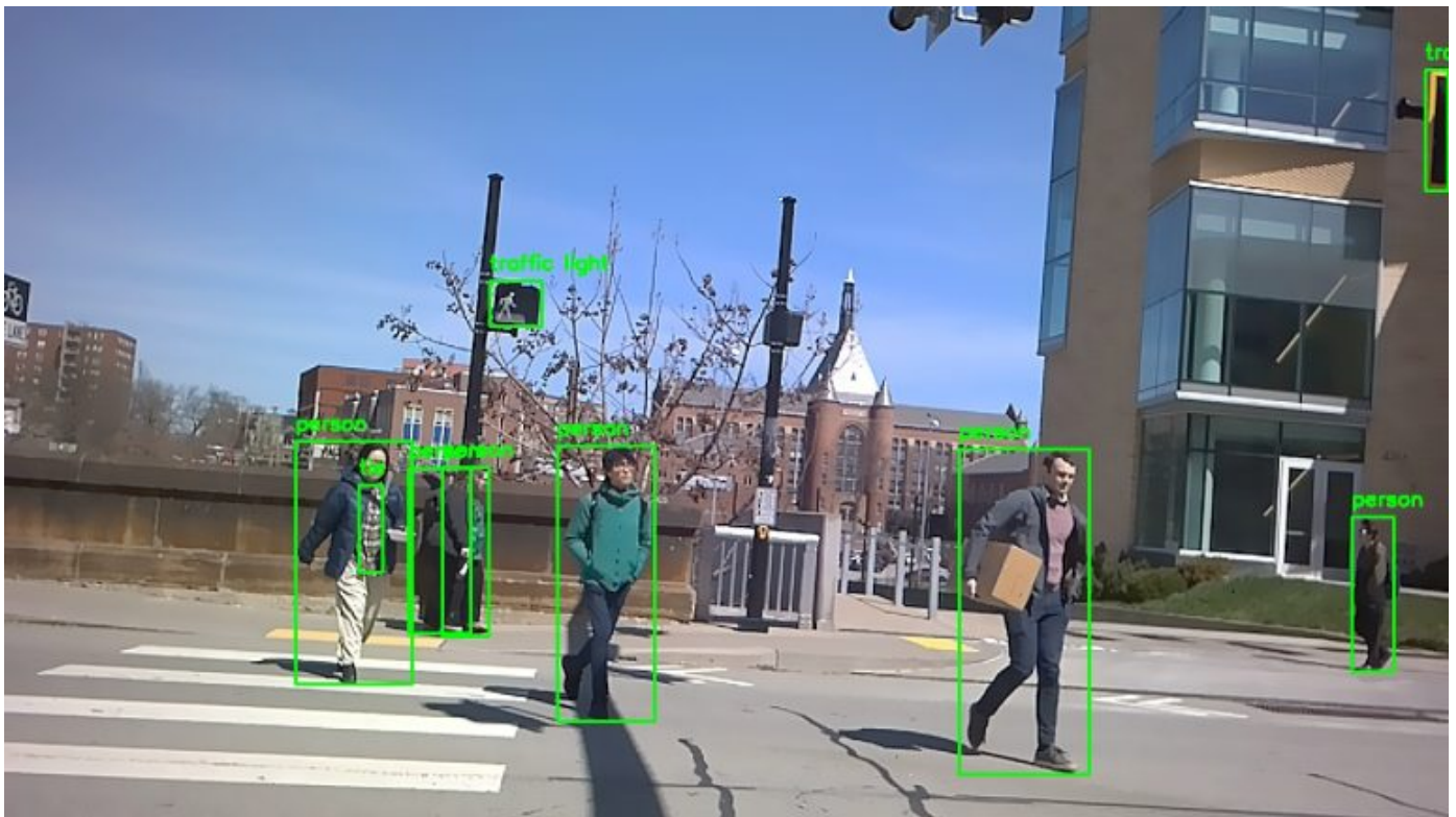
Figure 12: Bounding boxes on an input image that was used during testing. We observe that not only are the locations correct, but the classifications of the objects are completely correct.
