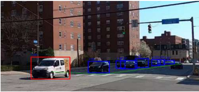
Fig. 6. An example frame from the Fifth and Craig intersection, with the lane boundaries marked in green. The cars included in the vehicle count are boxed in blue, while the cars not included in the vehicle count are boxed in red.
