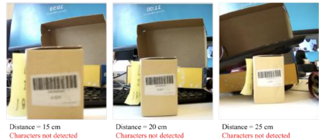
Fig. 4. OCR Distance test with TedGem 1080P WebCam.
