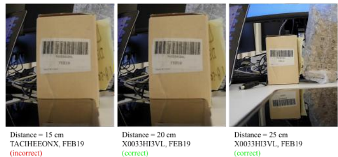
Fig. 5. OCR Distance test with NexiGo N60 1080P WebCam.
