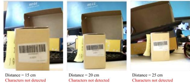
Fig. 4. OCR Distance test with TedGem 1080P WebCam.
