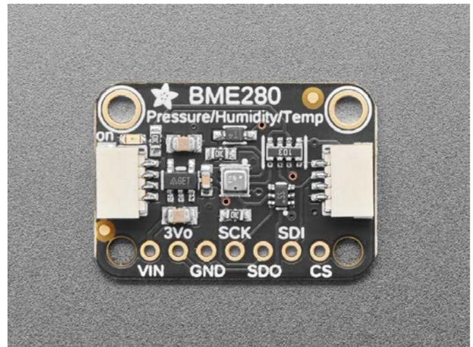
Fig. 7. Adafruit BME280 sensor [5]
