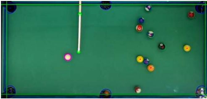
Fig. 4. Cue stick detection shown on the image.
