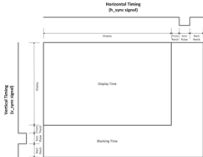
Figure 3: A diagram of the VGA timing specification
