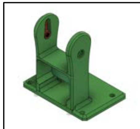
Figure 11. Isometric View of new OAK-D SR Mount. 3D-Printed elements are in Green.
