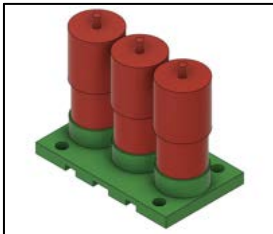
Figure 19. Pump Holder. 3D-Printed elements are in Green, and electronics are in Red.
