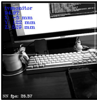
Figure 9. Sample Depth Camera output from OAK-D SR.
